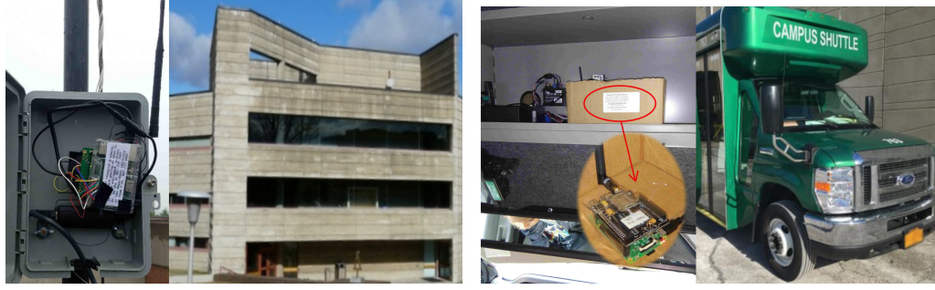
(a) LoRa base station installed on a roof. (b) LoRa end device installed on a shuttle.
